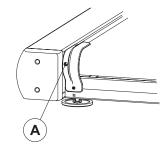
**NOTE:** Do not exceed one full turn of the adjusting screws in either direction. If, after one full turn, the belt does not track properly, contact Customer Support Services. The phone numbers are listed in Section 6.7, titled How to Obtain Product Service.
